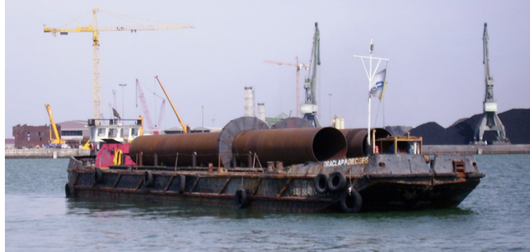
Figure 4: Auxiliary boat to transport materials from the coast to the floating platform. This boat also provided fresh water for slurry mixing, casings for the piles and reinforcement rebars. Other operations included tugging and transporting personnel from land to the platform and vice versa.
