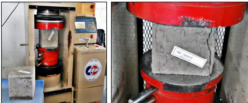
Figure 3a and 3b. Cube compression test
