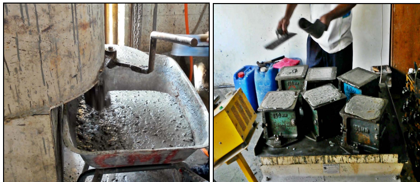
Figure 2a and 2b. Test 2 TM2 concrete collection and test cubes preparation
